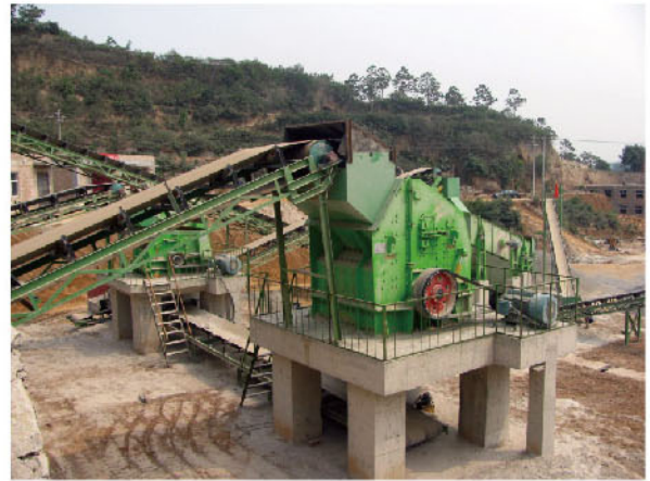
HC-579 反击式破碎机在加工砂石骨料 HC-579 impact crusher is producing aggregates
